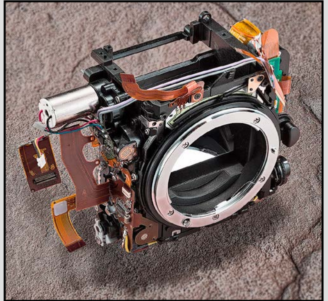
Figure 1: Nikon D750 mirror box. One of the DC motors is clearly visible on the upper left. Image: courtesy Professor Bob Newman.
