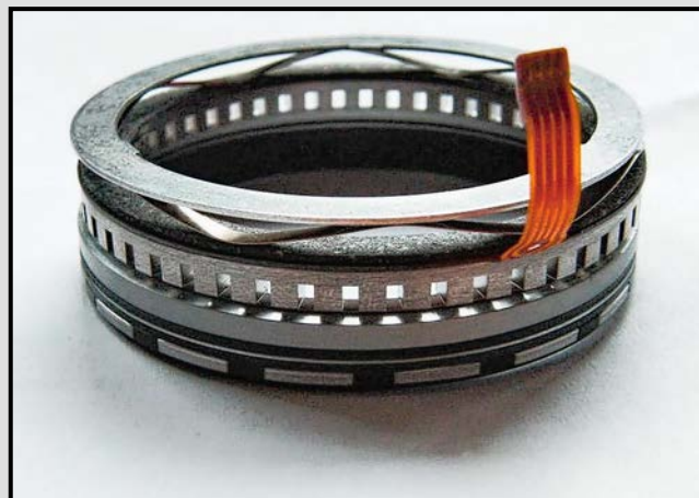
Figure 2: An ultrasonic motor: notice how the ring on top pushes a spring against the stator (with the teeth) so that it makes good friction contact with the rotor that sits underneath.
