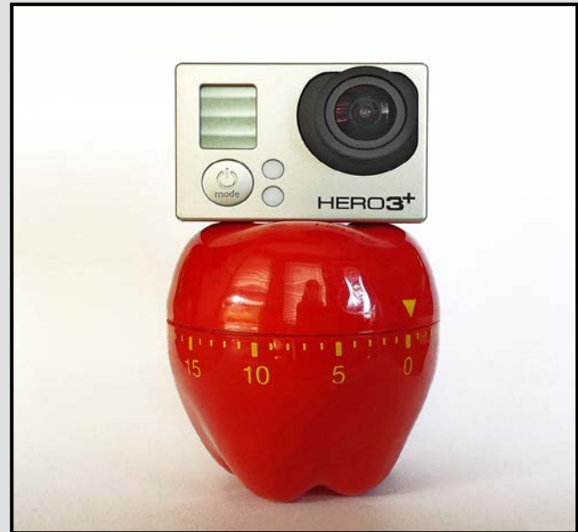
Figure 3: GoPro mounted on a kitchen timer slowly rotates as a time-lapse sequence is shot.
