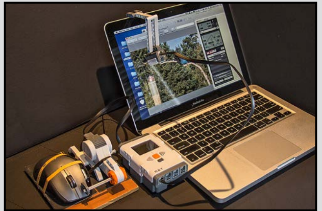
Figure 3: Light sensor pointed at the LiveView image detects the arrival of a bird and triggers the shutter via the wireless mouse.
